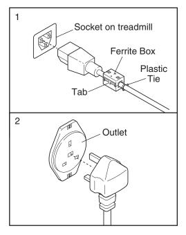
DANGER: Improper connection of the equipment-earthing conductor can result in an increased risk of electric shock. Check with a qualified electrician or serviceman if you are in doubt as to whether the product is properly earthed. Do not modify the plug provided with the product—if it will not fit the outlet, have a proper outlet installed by a qualified electrician.
